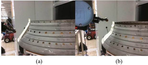
Figure 9: Inner linear taping. (a) No feedback. (b) Force feedback
